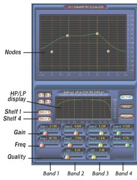
Parametric Equalizer with Shelf 1 and 4 on
